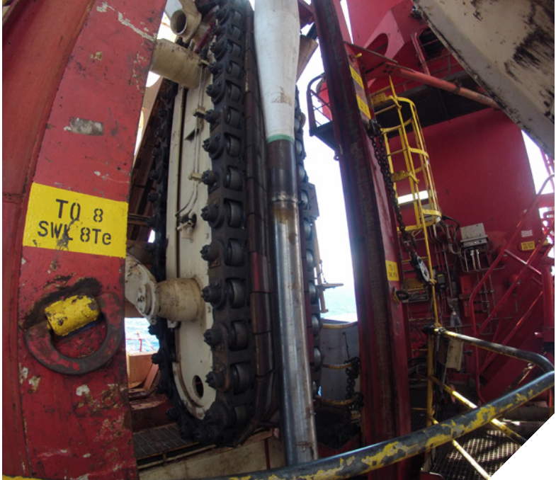
Transition pieces connect pipelines with varying cross-section, allowing greater utilization of reel capacity.
